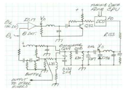
Figure 2. Portion of the IC-725 PLL Unit
