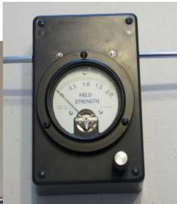
Figure 2. Modified Meter face with Sensitivity Control at lower right.
